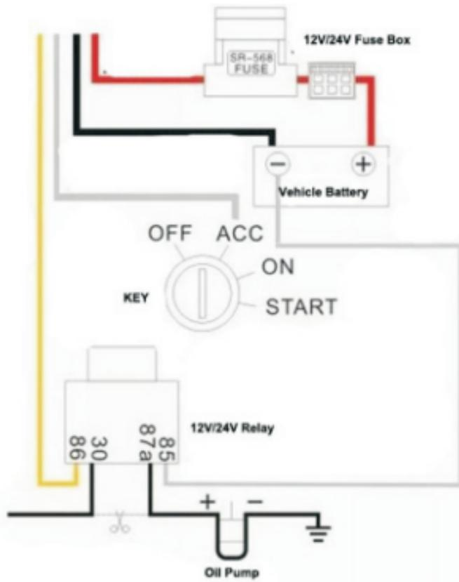
1. Power wire, ACC detection wire, Engine power or oil control relay wire (4pin)
